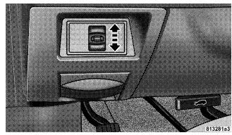
The power adjustable accelerator and brake pedals allow the driver to establish a comfortable position relative to the steering wheel and pedals.
